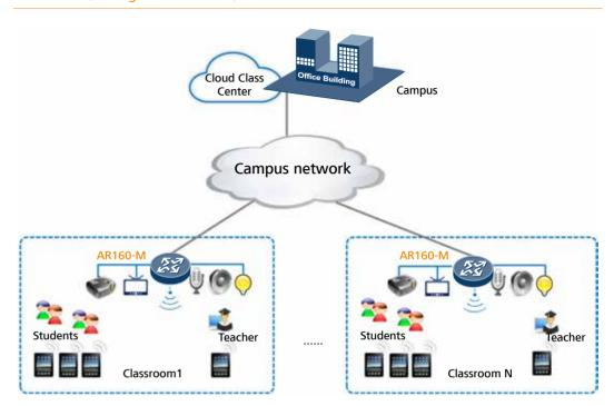
This illustration shows that the AR160-Ms can be deployed as CCE (Classroom Cloud Edge, the classroom cloud boundary) devices, to realize unified connection, centralized management, security accessing and intelligent controlling equipment in the classrooms, the AR160-Ms can support remote teaching, immediate feedback and other teaching applications.
