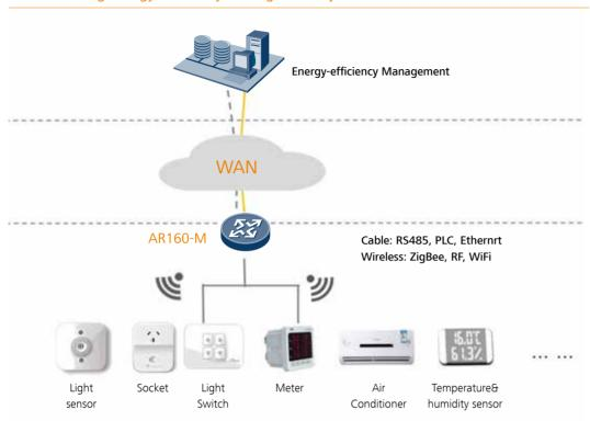
As IoT Gateways, this illustration shows that the AR160-Ms can connect many kinds of intelligent terminal equipments, such as lighting, air conditioning system meter device, sensor, controller meter in the buildings, to implement unified access, intelligent control and centralized management. The customers can experience intelligence building lighting, air conditioning environment and save energy cost.
